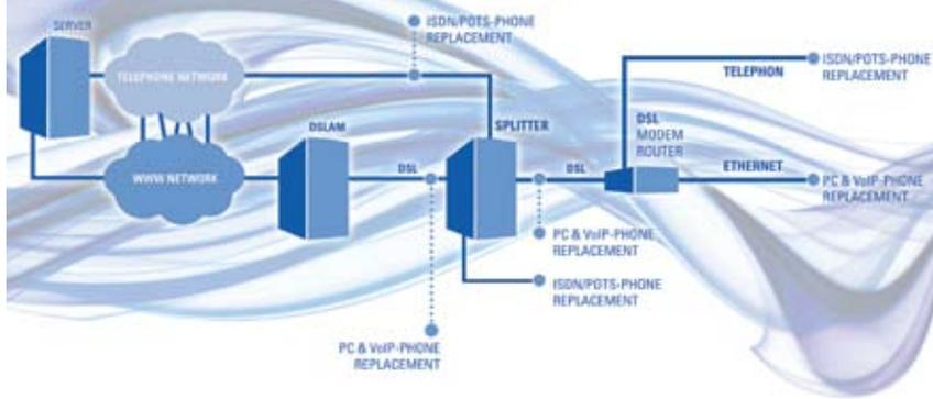
various telephone interfaces. A variety of testers are available which all support POTS and ISDN accesses as well as VoIP via Ethernet or xDSL.
